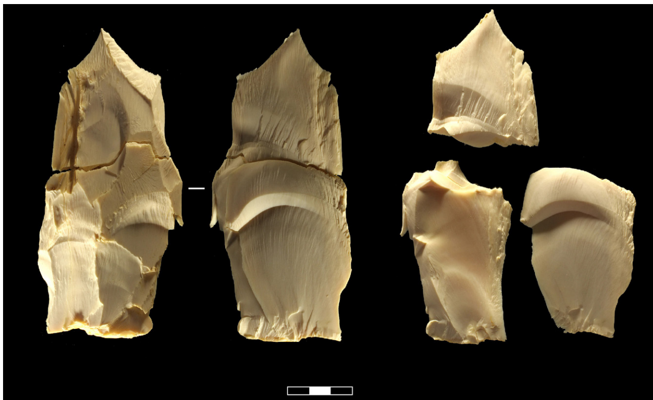
Fig. 21 – Ivory blade-like flake split into three pieces, removed by a single stroke from a mammoth tusk frozen up to -60^{\circ}\text{C} , experiment carried out in 2007.
